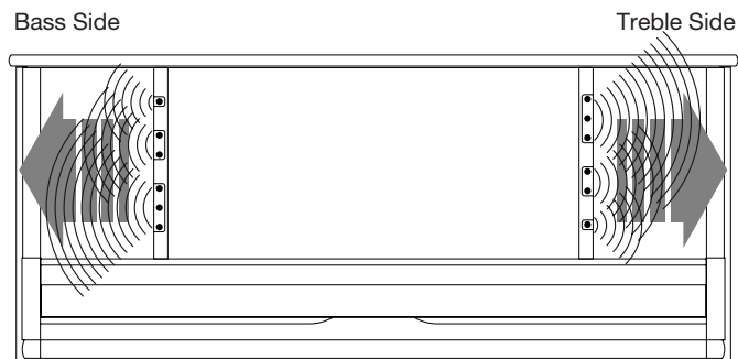
Inverse Tone Release System (K-6 and K-5)
